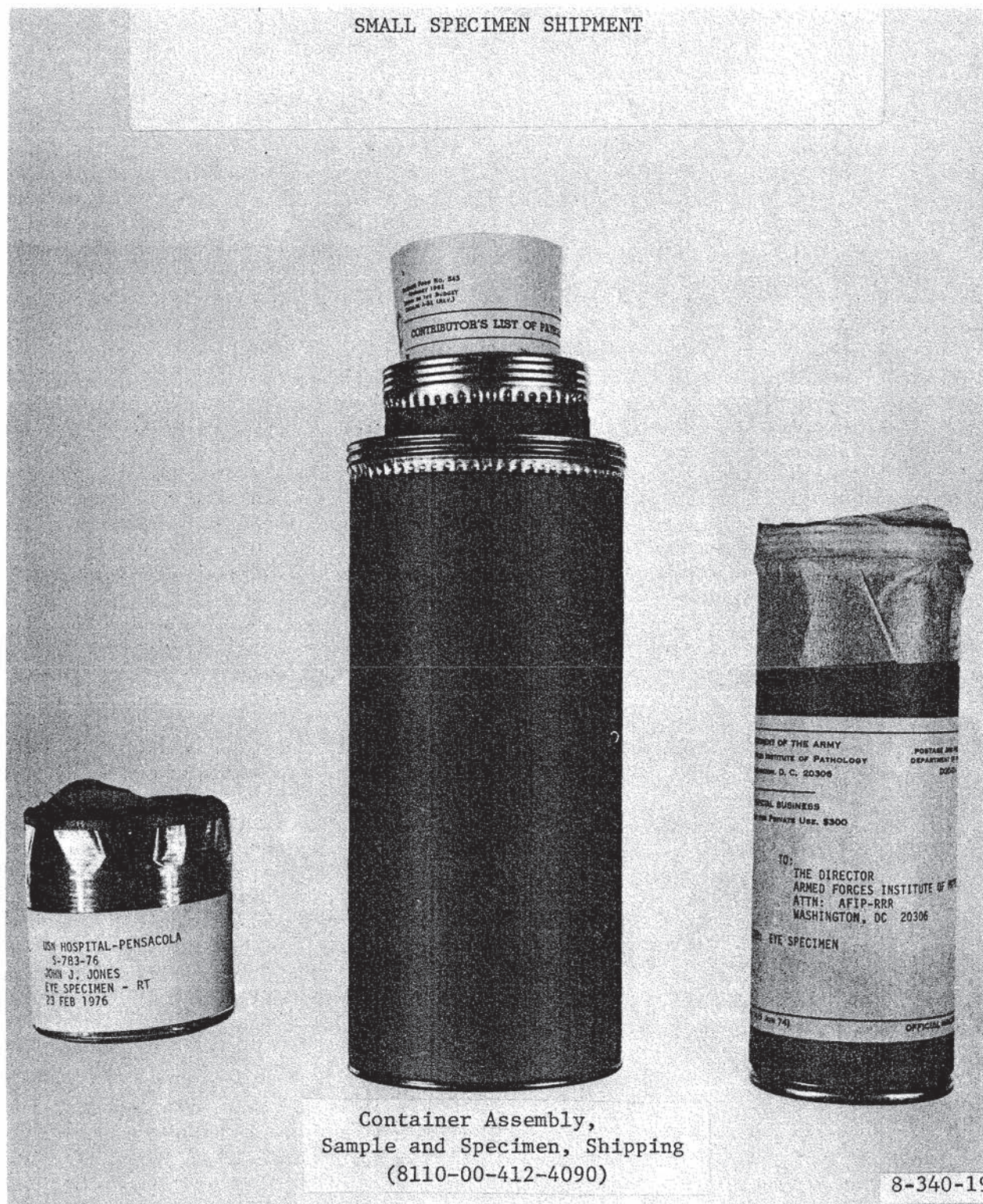
Figure 19. Small specimen shipping container.
