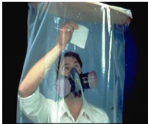
Figure C-1 IAA Fit Test Enclosure
