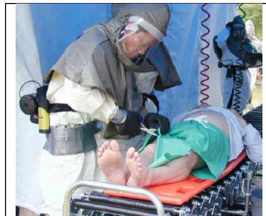
Figure D-24 Loose-Fitting CBRN PAPR
