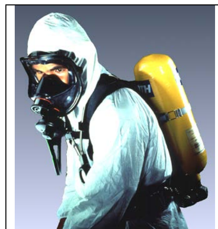
Figure D-2 Open-Circuit SCBA
