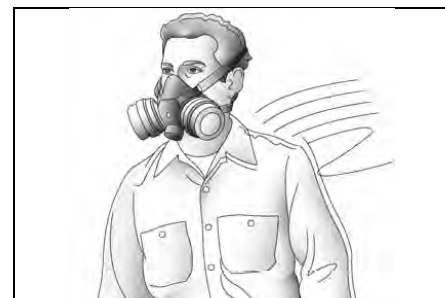
Figure D-10 Half Mask, Non-Powered, Air- Purifying Respirator
