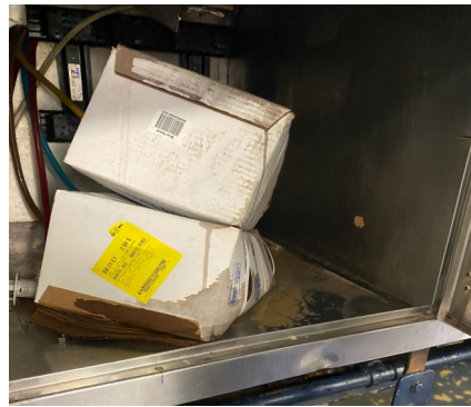
Fig.3. Cardboard box under galley beverage line soiled in water.
